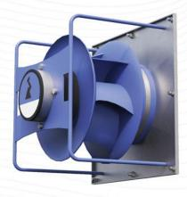
State-of-the-art eC fans of the latest generation regulate the required air output for supply and exhaust air as required. The control and regulation of the device takes place via a DDC system with self-optimizing mode of operation for the removal of moisture from the swimming pool.
